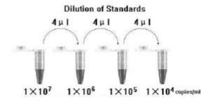
To generate a standard curve on the real-time system, all four dilution standards should be used and defined as standards with specification of the corresponding concentrations.
